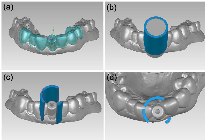
**FIGURE 3** Design procedure of guide tube. (a) Axis feature of cylindrical passage. (b) Circular tube. (c) Lateral view of separate guide tube parts. (d) Top view of separate guide tube parts.
