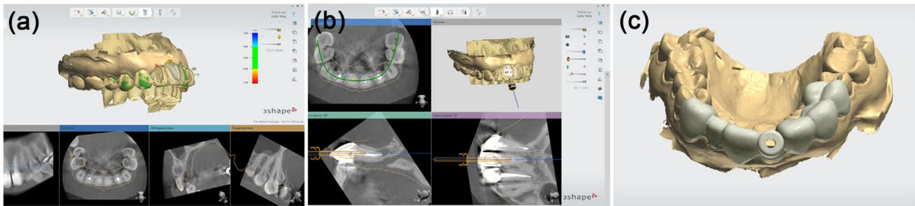
**FIGURE 2** Design procedure of guide prototype. (a) Superimposed surface and volume data. (b) Placement of virtual fixation pin. (c) Designed guide prototype.
