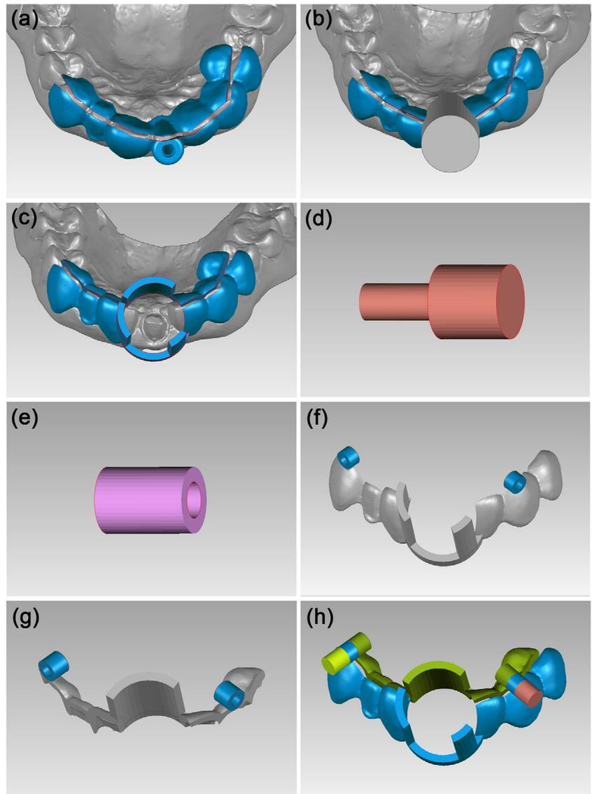
**FIGURE 5** Designed adaptors. (a) Top side view of the adaptor of turbine handpiece. (b) Bottom side view of the adaptor of turbine handpiece. (c) Top side view of the adaptor of electric handpiece. (d) Bottom side view of the adaptor of electric handpiece.
