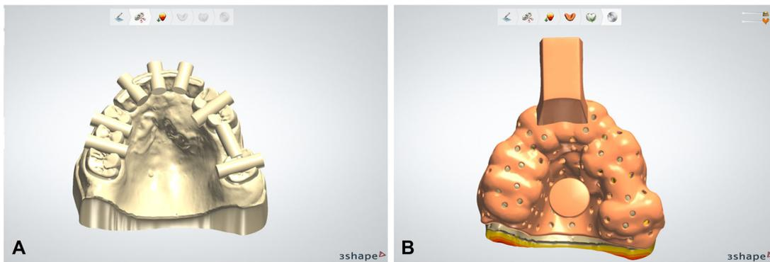
**Figure 6** Design the individual full arch tray with a dental CAD software. A, Combined data of the dentition and the inserted segmental individual tooth trays. B, Design of individual full arch tray.
