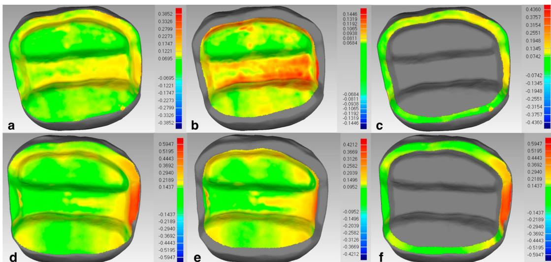
**Figure 5.** Colour-coded difference images showing the fitness of different groups. (a) Overall gap of Group DI; (b) internal gap of Group DI; (c) marginal gap of Group DI; (d) overall gap of Group CI; (e) internal gap of Group CI; and (f) marginal gap of Group CI.
