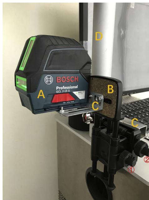
**Fig 1.** The 2-plane leveling and alignment lasers and the fixing and adjusting devices: **A**, orthogonal laser; **B**, 2-way focusing adjuster; **C**, customized connectors; **D**, the pole of SLS machine; **1**, up and down adjustment knob; **2**, left and right adjustment knob.
