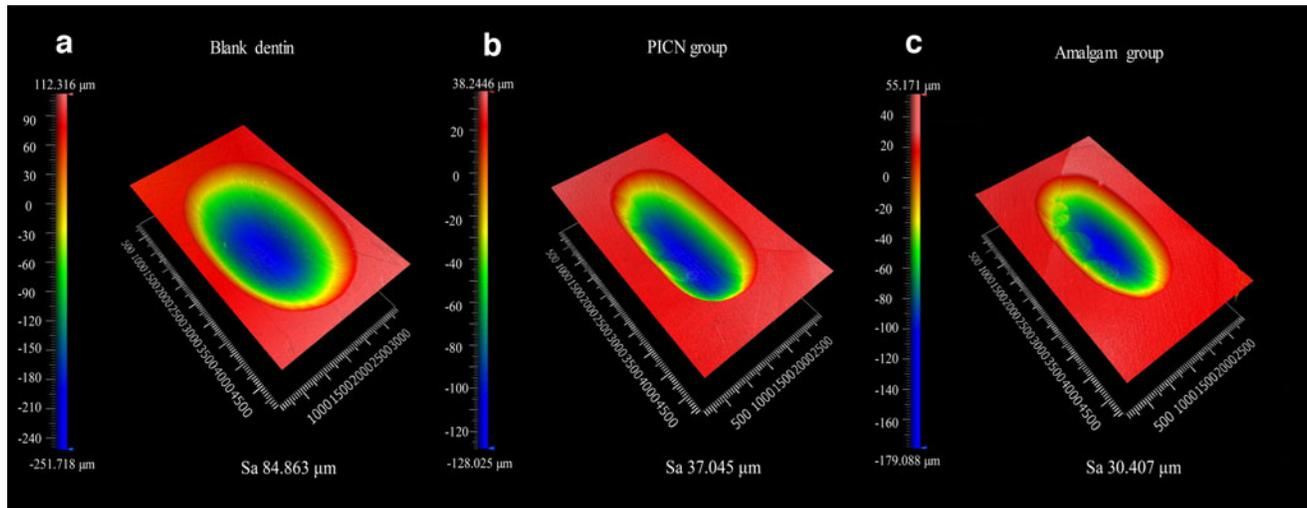
**FIG. 5.** Three-dimensional morphology of wear scars in the blank dentin (a), PICN group (b), and amalgam group (c). PICN, polymer infiltrated ceramic network.
