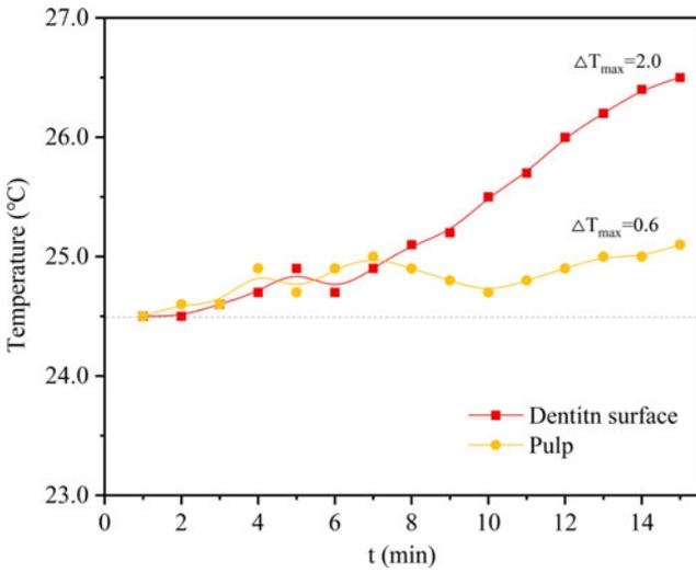
**FIG. 3.** The rise of temperature of dentin surface and pulp during the fs-laser processing.
