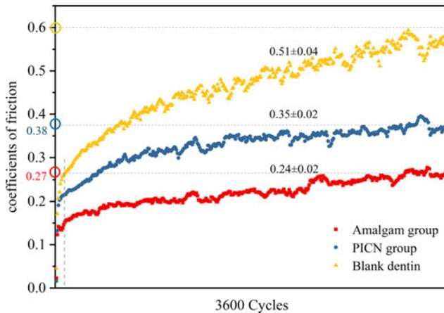
**FIG. 4.** Coefficients of friction during 3600 cycles for the three friction pairs.
