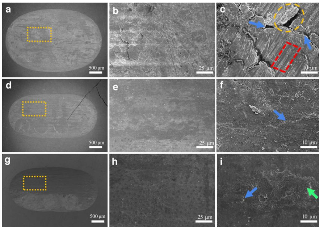
**FIG. 6.** Morphologies of the wear scars in the three friction pairs. From left to right, the three columns show the wear mode of dentin at magnifications of 30×, 600×, and 2000× in the three friction pairs. From top to bottom, three rows indicate blank dentin (a–c), dentin in the wear scar of PICN group (d–f), and dentin in the wear scar of amalgam group (g–i), respectively.
