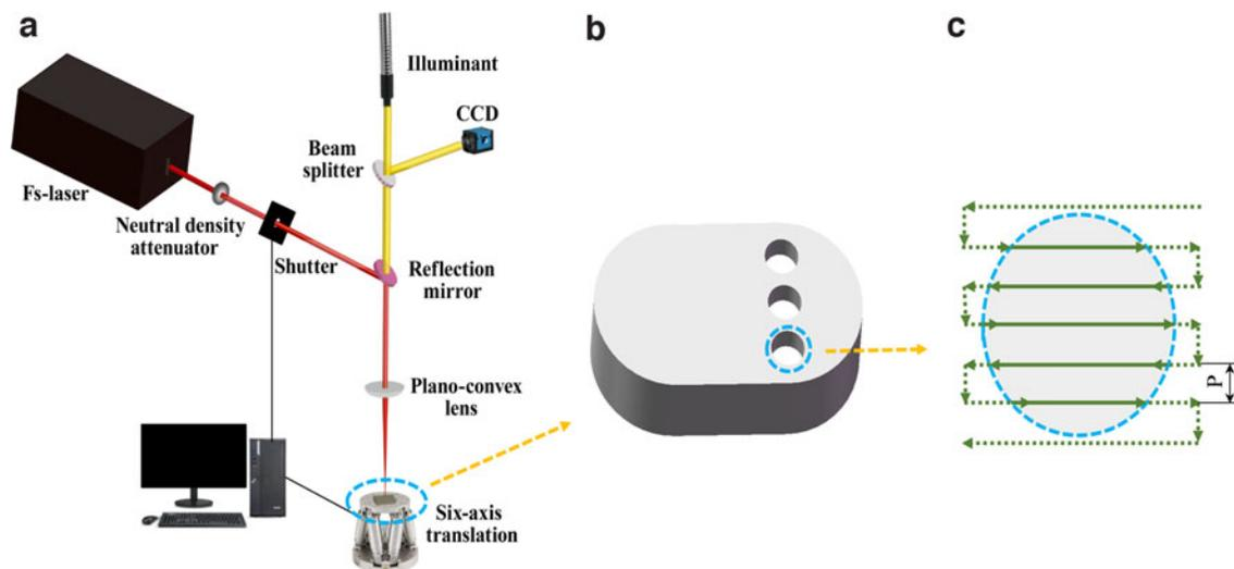
FIG. 2. Scheme of the fs-laser used for the ablation of the dentin samples (a). Dentin samples were placed on the translation. The scanning paths of fs-laser for microcavity preparation are shown in b and c. fs-laser, femtosecond laser.
