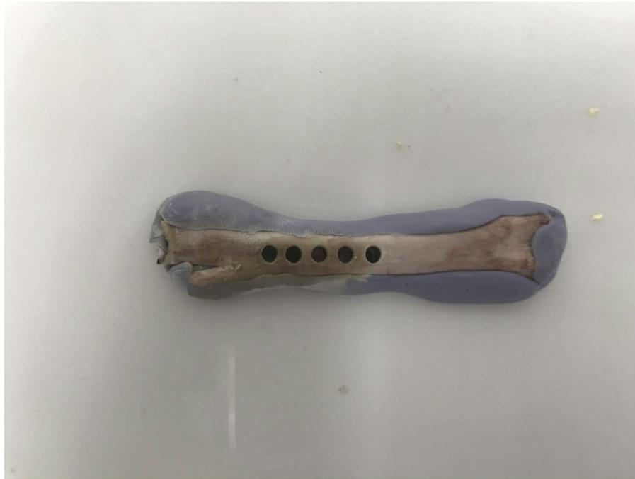
**Fig. 4.** Implant cavities prepared with different combinations of laser-cutting parameters.
