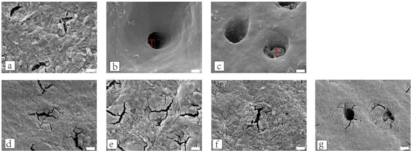
**Fig. 4** a, b, c, d, e, f, g Scanning electron microscopy of dentin after the surfaces were conditioned with water, 35% phosphoric acid for 15 s, SE-Bond for 20 s, 2 wt% EDTA, 1% (v/v) acetic acid, 1wt%
