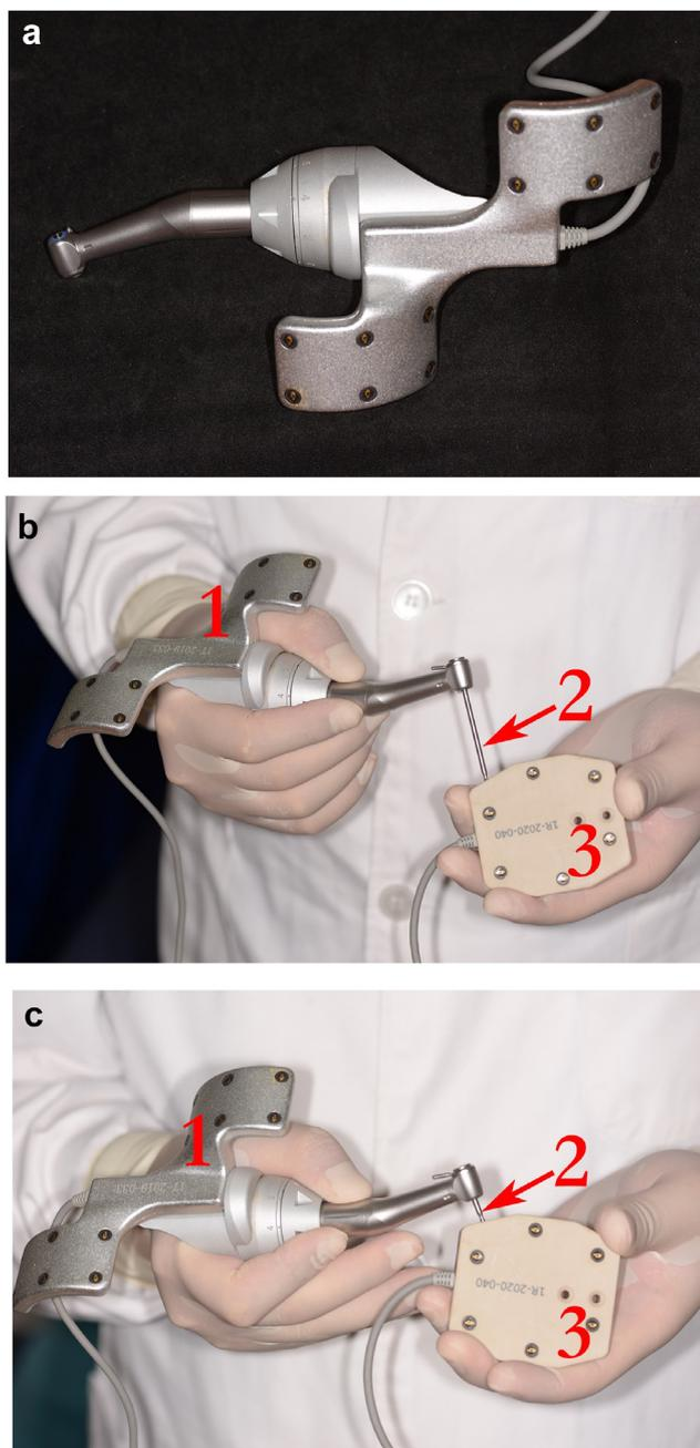
**Figure 2.** a. An adjustable handpiece with five gears. b. Calibrating the adjustable handpiece with a long drill using a handpiece-locating device and a reference device before the dental implant surgery. 1 - handpiece-locating device; 2 - long drill; 3 - reference device. c. An adjustable handpiece with a short drill. 1 - handpiece-locating device; 2 - short drill; 3 - reference device.
