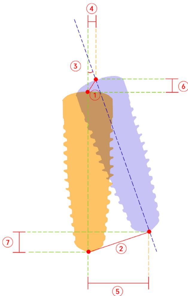
**Figure 8.** Deviations between the preoperative (planned, orange implant) and postoperative (actual, blue implant) implant positions. ① Entry-point deviation; ② Apical-point deviation; ③ Angular deviation; ④ Entry-point horizontal deviation; ⑤ Apical-point horizontal deviation; ⑥ Entry-point depth deviation; ⑦ Apical-point depth deviation.
