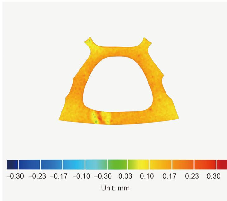
**Figure 8** 3D color-coded mapping of 3D deviation between intaglio surface of overall area of built specimen and that of design data
