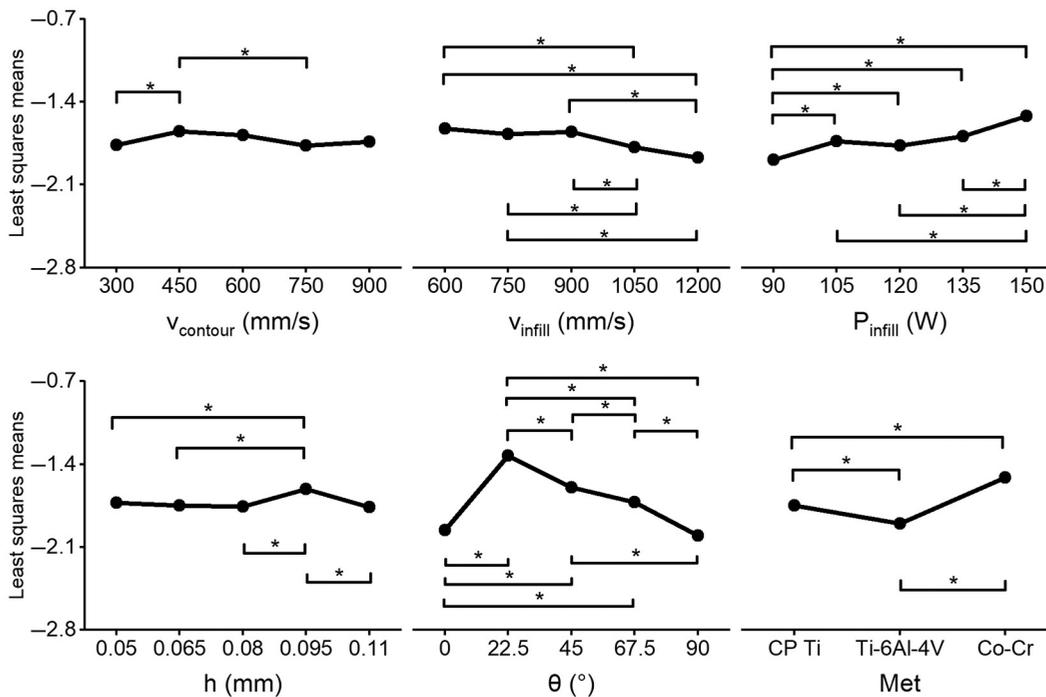
Notes:  $v_{\text{contour}}$ , contour scan speed;  $v_{\text{infill}}$ , infill scan speed;  $P_{\text{infill}}$ , infill laser power;  $h$ , hatch space;  $\theta$ , build orientation; Met, metallic powder type. \*Mean difference significant ( $P < 0.05$ )
