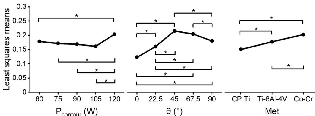
Notes:  $P_{\text{contour}}$ , contour laser power;  $\theta$ , build orientation; Met, metallic powder type. \*Mean difference significant ( $P < 0.05$ )
