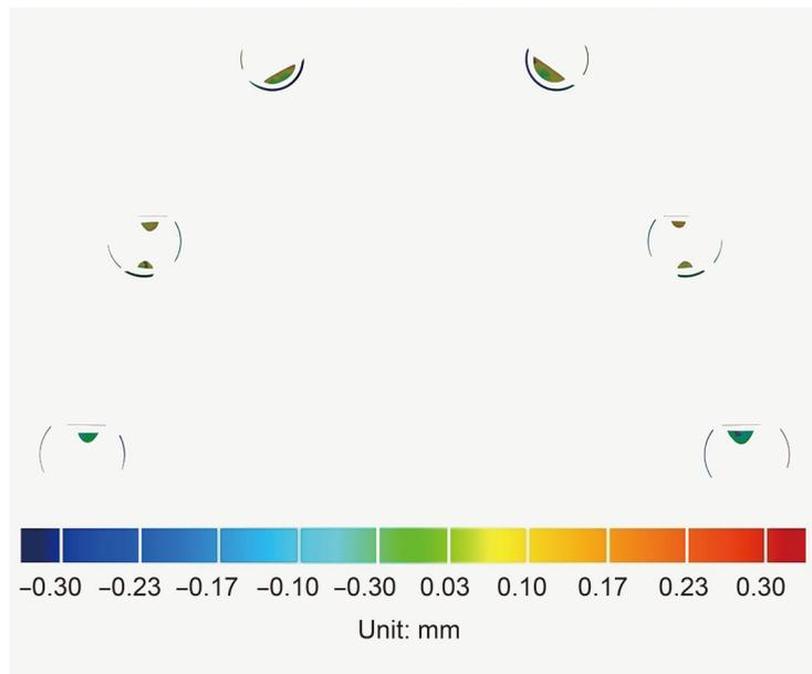
**Figure 7** 3D color-coded mapping of 3D deviation between intaglio surface of major connector area of the built specimen and that of design data
