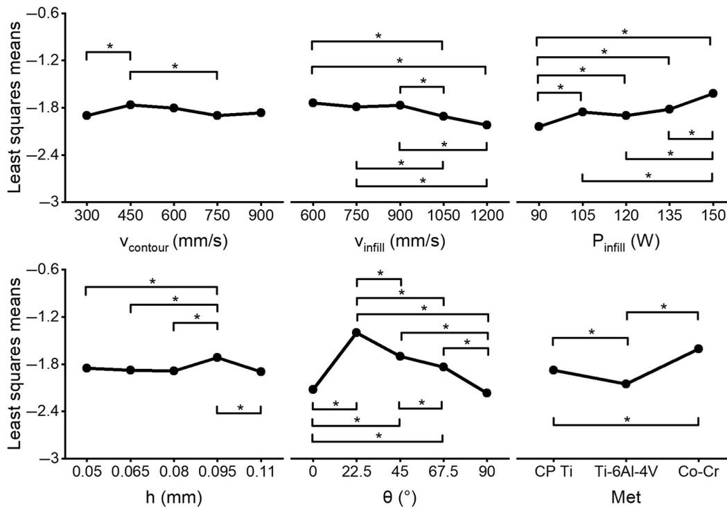
Notes:  $V_{\text{contour}}$ , contour scan speed;  $V_{\text{infill}}$ , infill scan speed;  $P_{\text{infill}}$ , infill laser power;  $h$ , hatch space;  $\theta$ , build orientation; Met, metallic powder type. \*Mean difference significant ( $P < 0.05$ )
