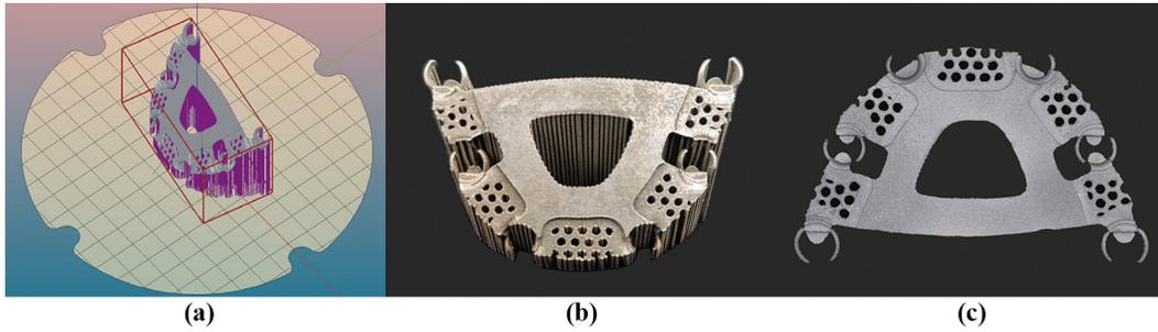
**Notes:** (a) Support generation; maxillary RPD framework specimen before removal of supports (b) and (c) after grinding and sandblasting
