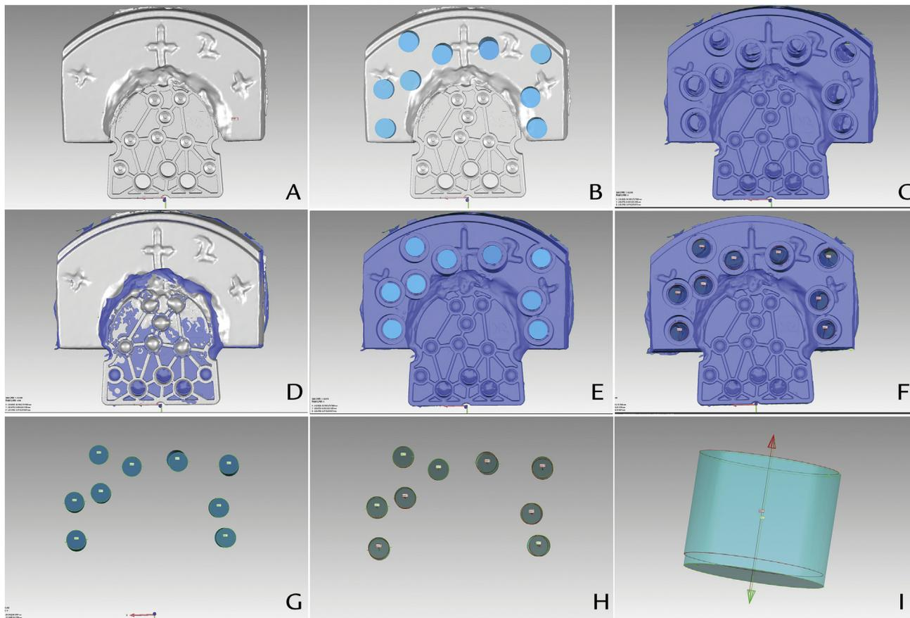
**Figure 5.** Accuracy evaluation process: A, Digitized radiographic guide imported into imaging analysis software program. B, Virtual implant planning and digitized radiographic guide in same coordinate system. C, Digitized surgical guide with actual milled sleeve bore holes imported into coordinate system. D, E, Digitized guides before and after milling superimposed by using characteristic grooves on surface of resin plate.
