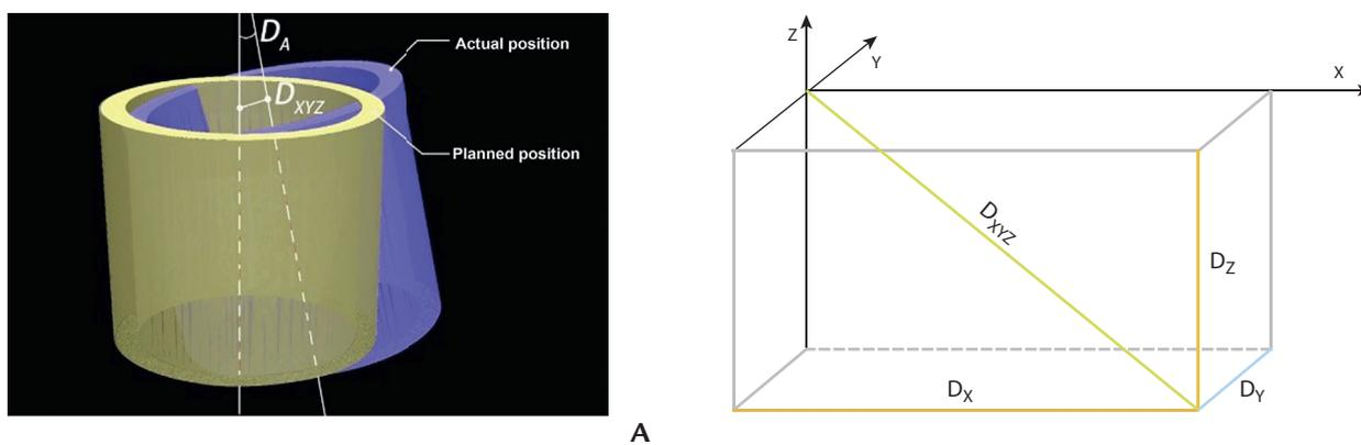
**Figure 6.** Deviation of sleeve reference points and axis angle. A, Global linear deviation in 3D coordinates ( $D_{XYZ}$ ) and angular deviation ( $D_A$ ). B, Linear deviations of surgical guide sleeves reported as  $D_x$ ,  $D_y$ , and  $D_z$  in 3 directions of x, y, and z.
