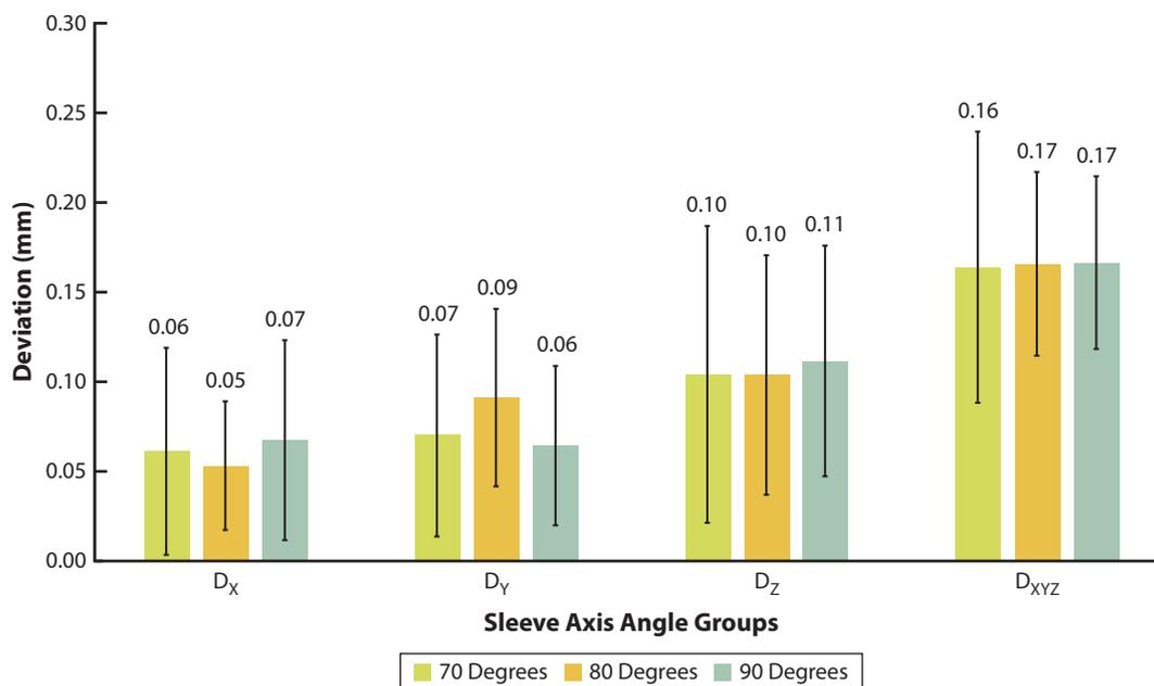
**Figure 8.** Mean deviations of sleeve bore holes in 3 sleeve axis angle groups (70, 80, 90 degrees). D<sub>x</sub>, D<sub>y</sub>, D<sub>z</sub> represent deviation in x, y, and z directions, and D<sub>xyz</sub> represents 3D global deviation.
