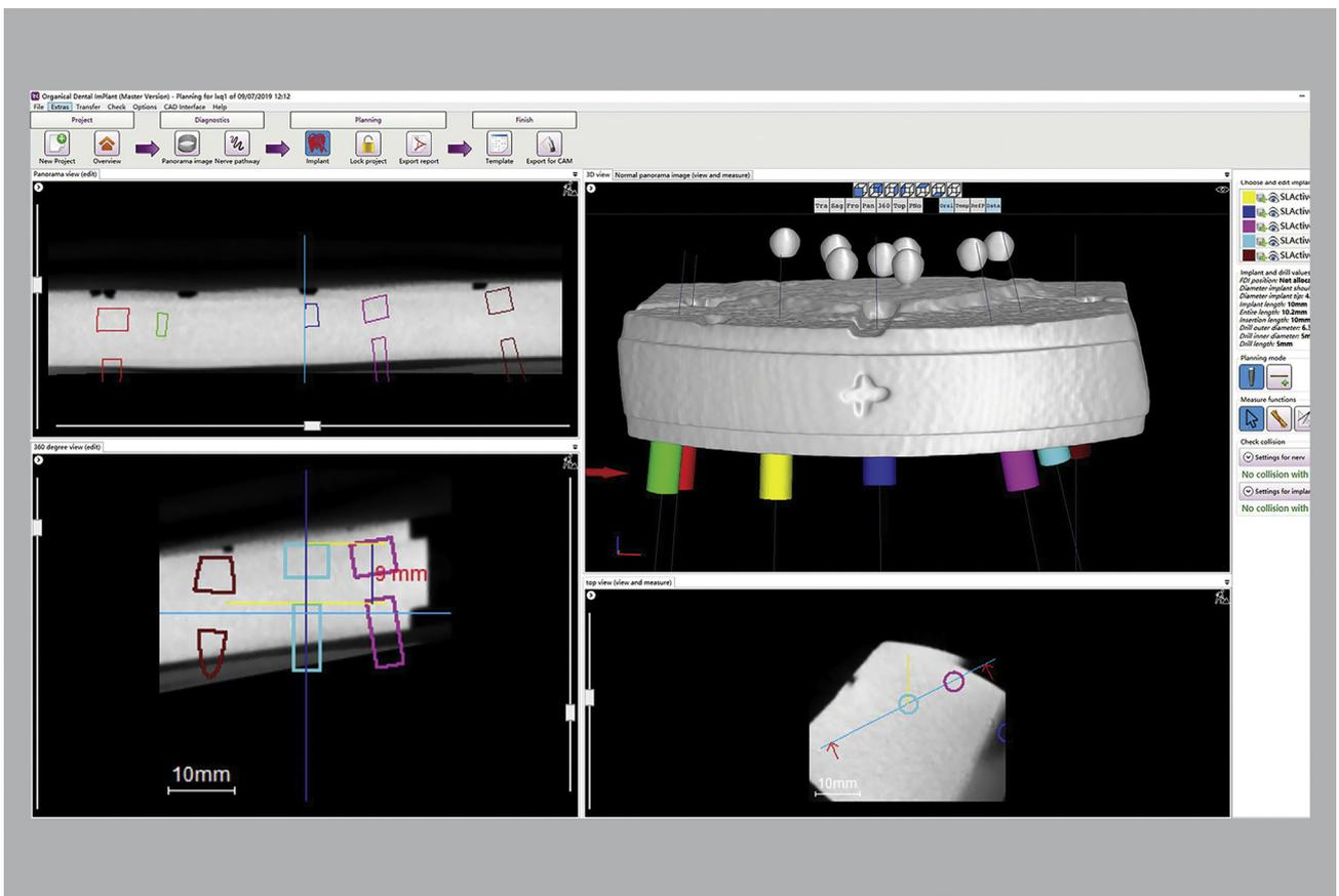
Figure 2. Positions of implants and sleeves virtually planned.
