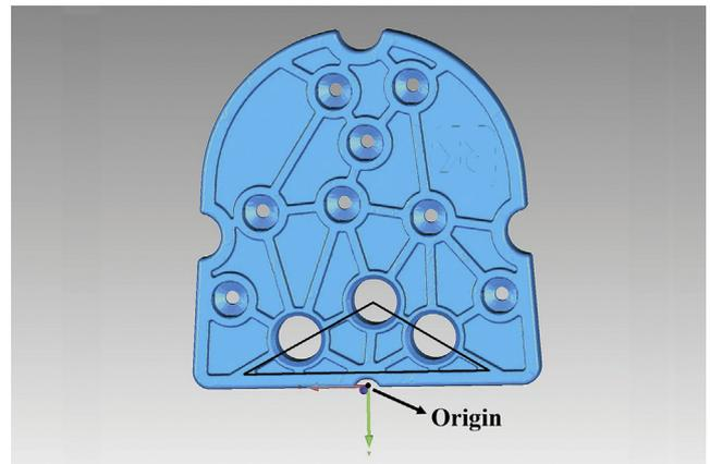
**Figure 4.** Origin of 3D coordinate set at middle point of straight border of diagnostic template.
