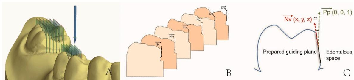
Fig. 5. Evaluation of angle between the prepared guiding plane (test) and the designed path of placement. A, Creation of six cross-sections parallel to the path of placement for each guiding plane. B, The direction vector ( $\vec{Nv}$ ) of guiding plane preparation on each cross-section. C, Measurement of angle ( $\alpha$ ) between the direction vector of prepared guiding plane ( $\vec{Nv}$ ) and the vector ( $\vec{Pp}$ ) of the path of placement on each cross-section.
