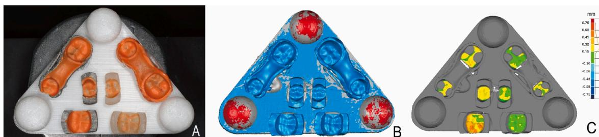
Fig. 3. Internal adaptation assessment of CAD-CAM guides. A, Internal gaps replicated by impression material. B, Three hemispheres were selected for aligning 2 scanning data. C, Internal gap thickness was assessed using 3D-compare analysis.
