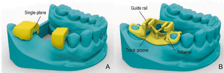
Fig. 2. Two types of guiding structures of CAD-CAM guides. A, Single-plane guiding structure. B, Triple-constraint guiding structure.
