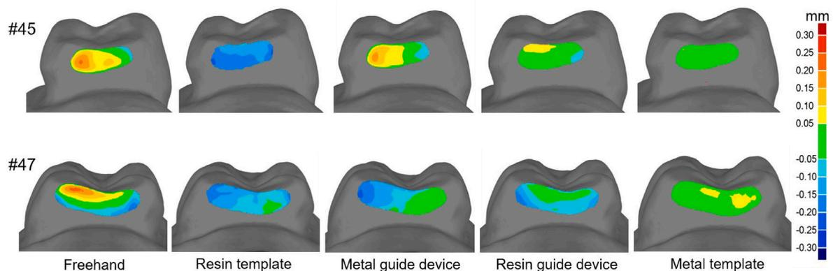
Fig. 6. Representative color-coded maps of 3D deviation of 3D trueness of guiding plane preparation. Green: deviation  $\leq 50 \mu\text{m}$ . Yellow through red: inadequate preparation. Cerulean blue through dark blue: excessive preparation.
