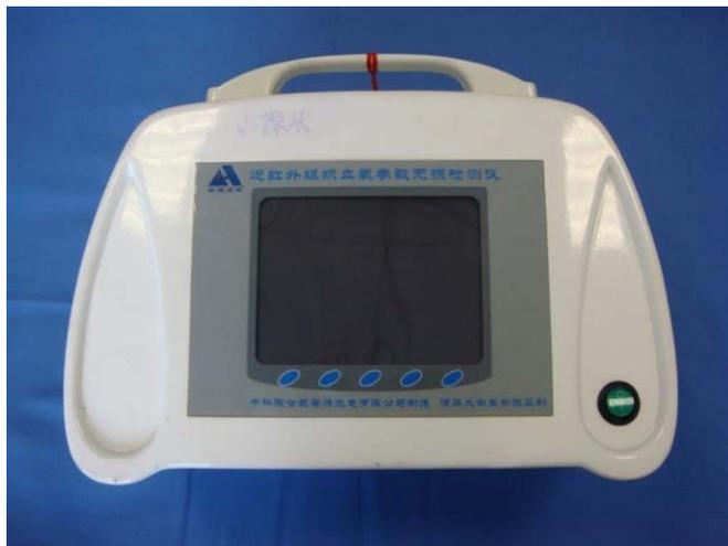
FIGURE 1. Near-infrared spectroscopy oximeter: TSAH-100.
