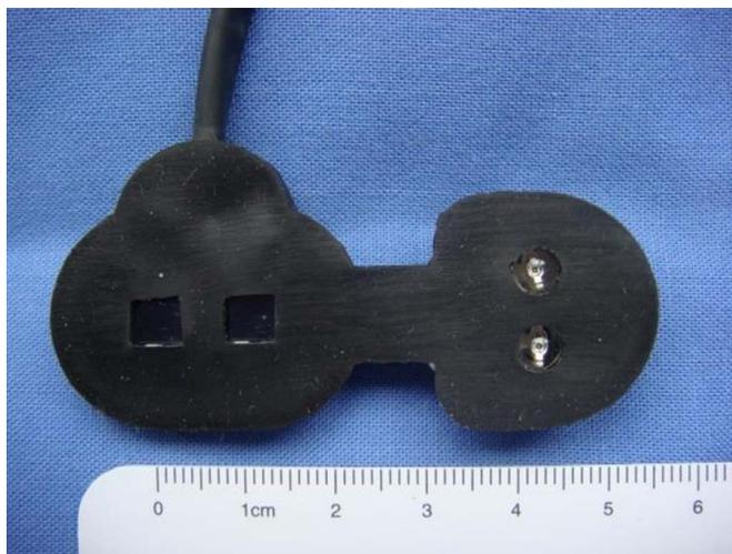
FIGURE 2. The TSAH-100 sensor is composed of a dual-wavelength near-infrared light source and 2 detectors, with distances of 3.0 and 4.0 cm, respectively, between the source and the detector.
