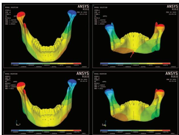
FIGURE 6. Nephograms showing transverse displacement in models A (top) and B (bottom). The two-dimensional fixation model showed displacement in the symphyseal fracture (indicated by an arrow) and the mandible tended to widen.
