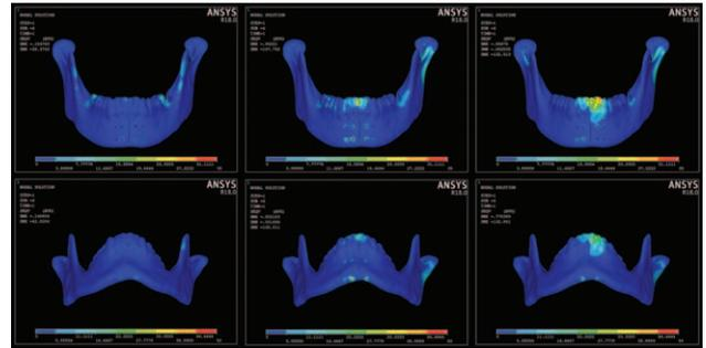
FIGURE 2. Stress distribution in mandibular models during intercuspal position (left), right unilateral molar clenching (middle), and incisal clenching (right).
