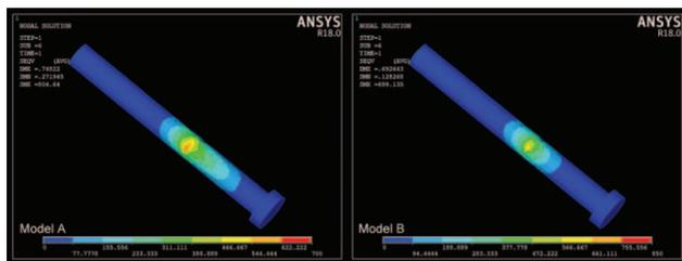
FIGURE 5. Stress distribution of the condylar long screw. The 2D fixation model (left) showed an area of high stress (red) and a wider range of stress distribution.
