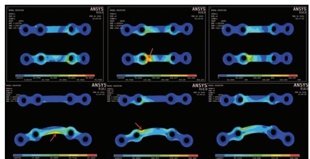
FIGURE 3. Stress distribution in plates during intercuspal position (left), right unilateral molar clenching (middle), and incisal clenching (right) in models A (top) and B (bottom). The arrows indicate stress concentrations.
