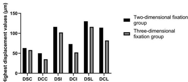
FIGURE 7. Maximum displacement during various loading conditions. In the abbreviations the initial D denotes displacement; the following S or C, respectively denotes the symphyseal and condylar intracapsular fractures; and the final C, I, or L denotes central, incisor, and lateral occlusion, respectively.
