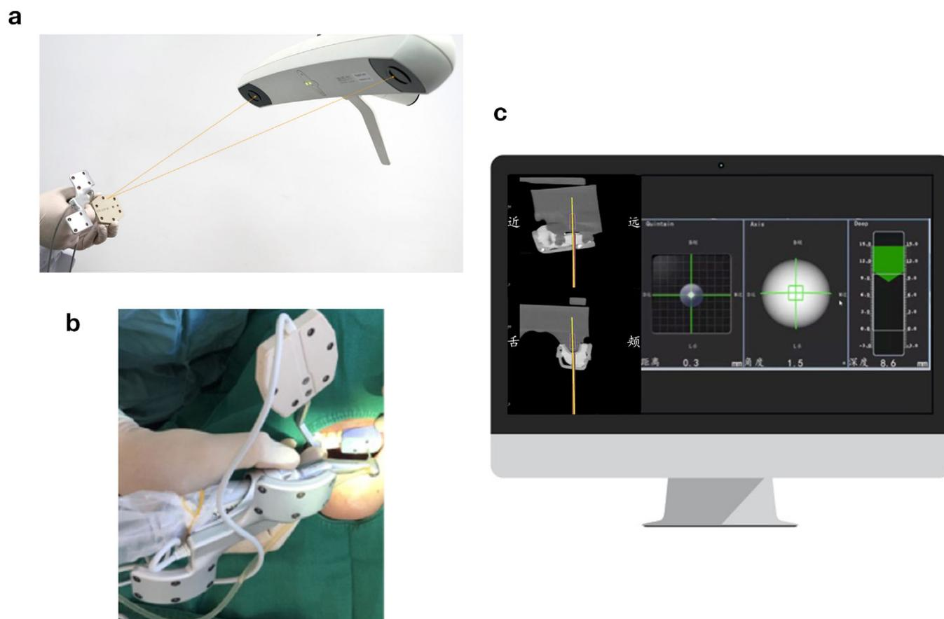
FIGURE 2 Training in placement of dental implants using dynamic navigation system. Video camera detection of the handpiece position through tags (A); video camera detection of the model position through markers (B); visual location of the drill and implant placement on the computer monitor (C)
