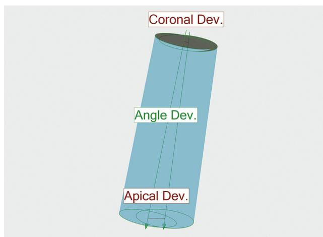
**Figure 5.** Implant deviation calculated based on reconstructed implant cylinders.
