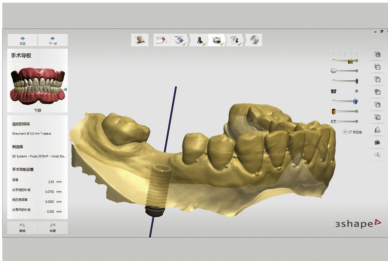
**Figure 1.** Surgical planning for implant surgery. Cone beam computed tomogram hidden to show implant position.
