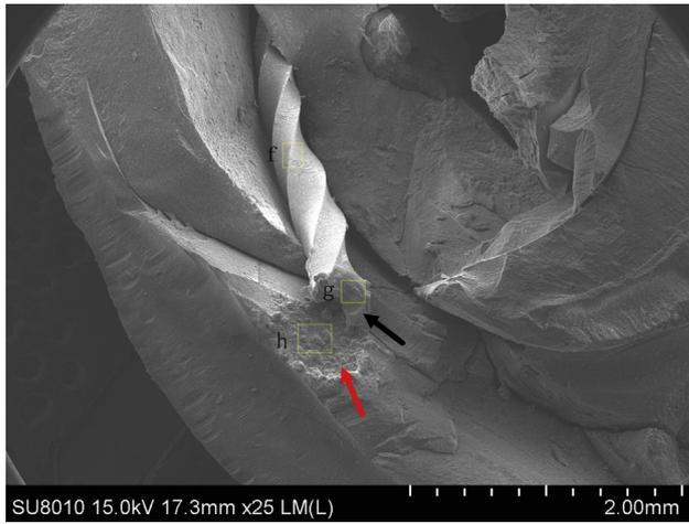
**FIGURE 6** – Scanning electron microscopy of the canal with the ProTaper Next X2 file after ablation. Dentin fusion (*red arrow*) and the file (*black arrow*). The energy-dispersive spectroscopic results of area f, g, and h are shown in [Figure 9](#).
