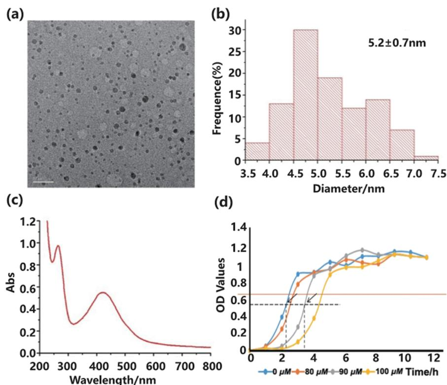
**Figure 1.** (a) TEM images of DNA-templated silver nanoparticles, the scale bar is 20 nm. (b) Histogram for particle size. (c) UV spectra for DNA-templated silver nanoparticles. (d) Effects of silver nanoparticles on *Enterococcus faecalis* growth.
