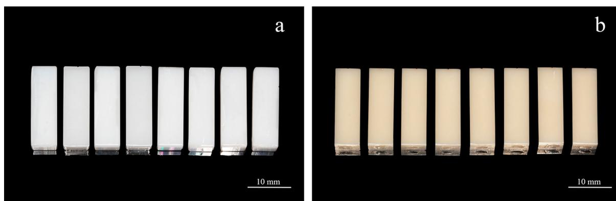
**Figure 1.** Two types of bar-shaped dental zirconia specimens. (a) SGZ specimens; (b) CZ specimens.
