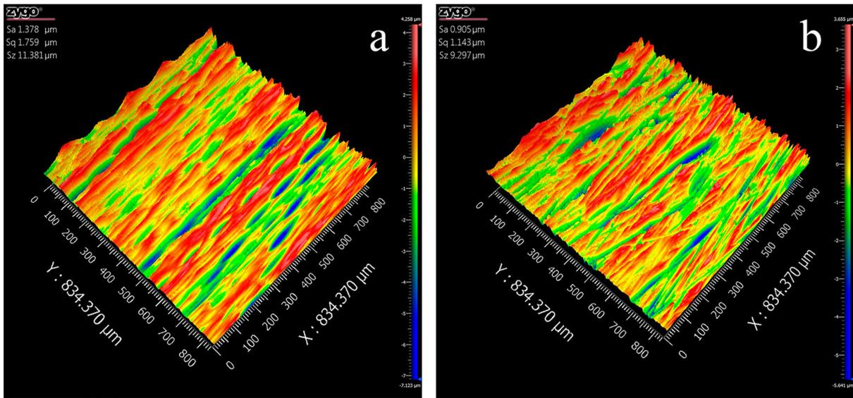
**Figure 5.** Surface area roughness (Sa) of CZ and SGZ specimens characterized by the white light interferometer. (a) Surface of CZ after grinding; (b) Surface of SGZ after grinding.
