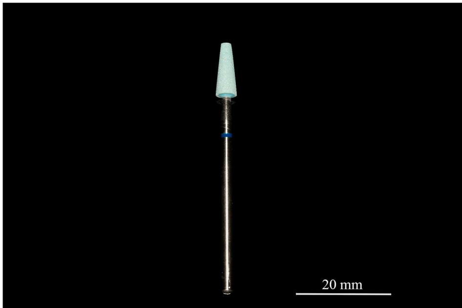
**Figure 2.** Ceramic diamond grinders used in this study.
