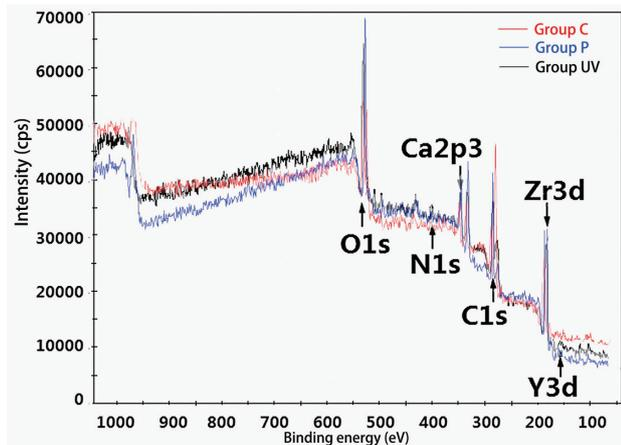
Fig. 4 XPS spectrum of zirconia in three groups.
