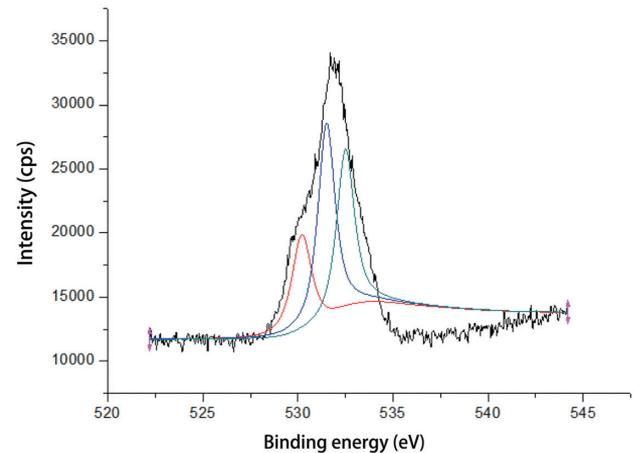
Fig. 5 The XPS O1s spectra of zirconia was fitted with three components. Dissolved (BE= $530.1 \pm 0.1$  eV), Oxide (BE= $531.2 \pm 0.1$  eV), and Hydroxide (BE= $532.5 \pm 0.2$  eV).
