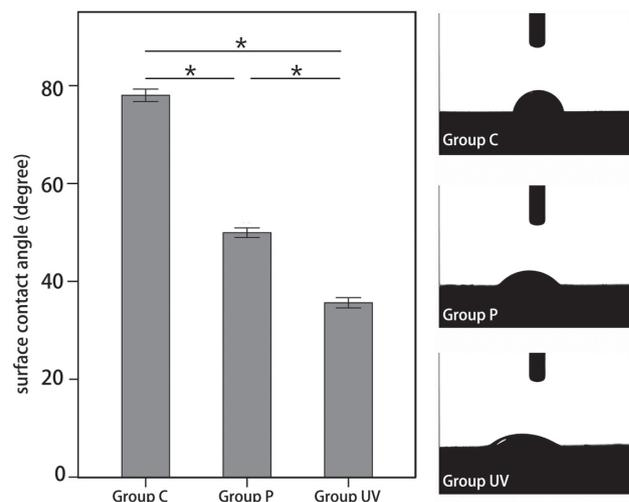
Fig. 3 After plasma and UV light treatment, the surface contact angles significantly decreased. Data are shown as mean $\pm$ SD ( $n=15$ )  $*p<0.05$ .
