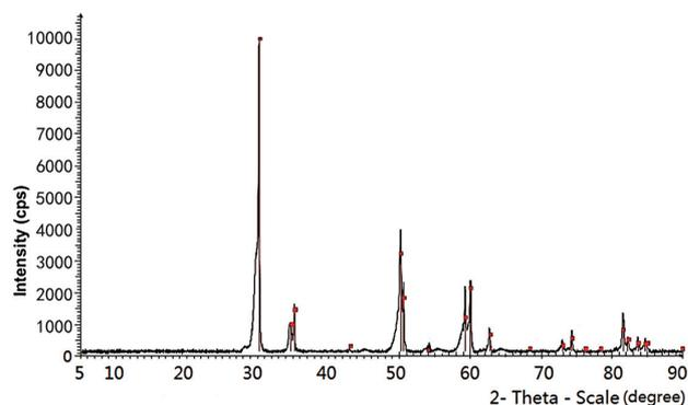
Fig. 2 XRD spectrum of zirconia disks. It is accord with zirconium yttrium oxide.
