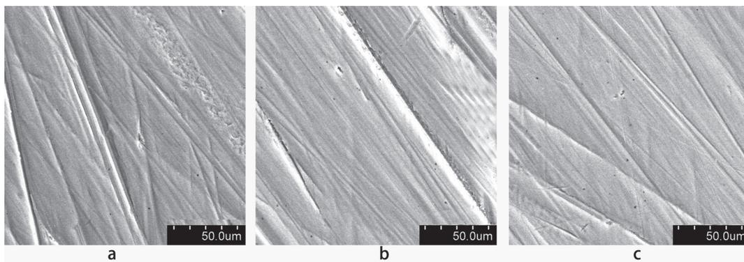
Fig. 1 Surface morphology of three groups of zirconia as SEM images. (a) Group C, (b) Group P, (c) Group UV.
