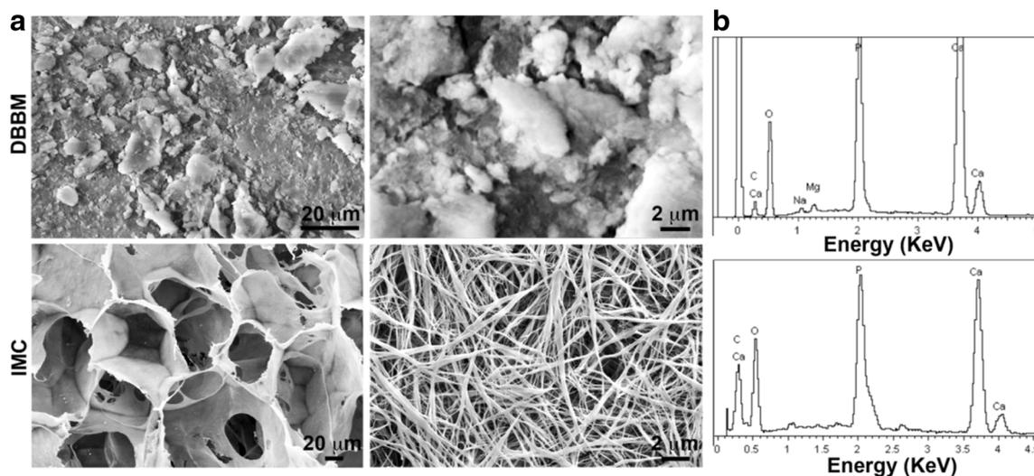
**Fig. 2** a Representative (left) low- and (right) high-magnification SEM images of DBBM and IMC. b EDS of DBBM and IMC
