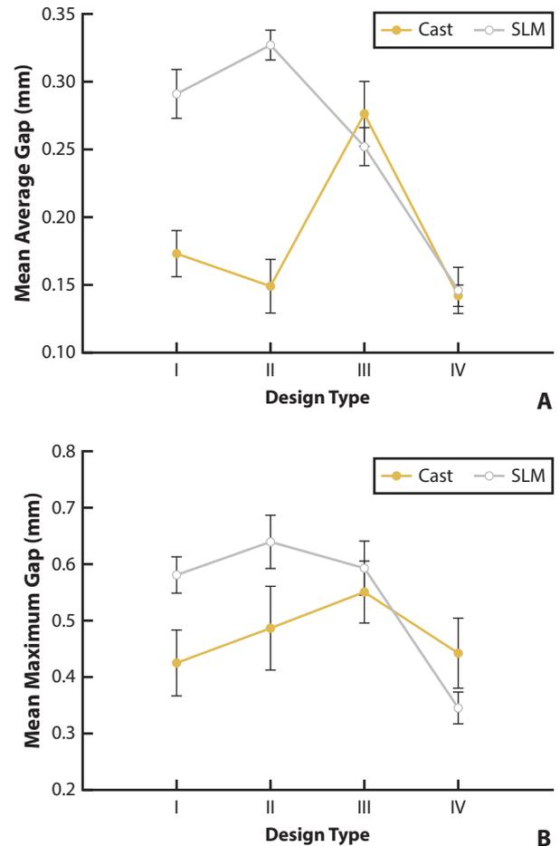
**Figure 4.** Influence of production methods and design types. A, Mean average gaps. B, Mean maximum gaps. Error bar indicates ±1 standard error. SLM, selective laser melting.
