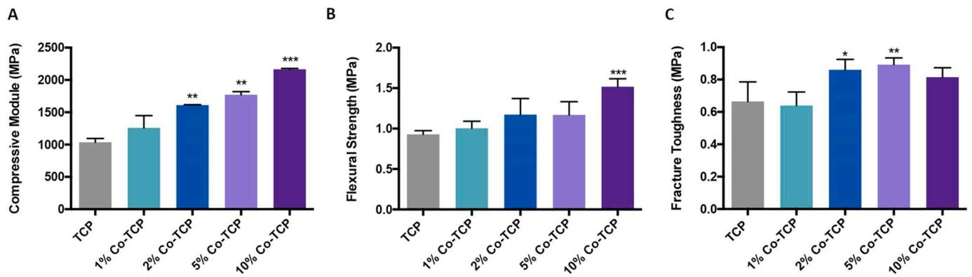
Fig. 3. Mechanical properties of Co-TCP with different concentrations of Co. (A) Compressive modulus. (B) Flexural strength. (C) Fracture toughness. \* $p < 0.05$ ; \*\* $p < 0.01$ ; \*\*\* $p < 0.001$  compared with pure TCP.
