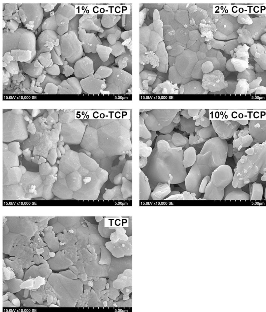
**Fig. 2.** SEM images showing the surface microstructure of TCP and Co-TCP ceramics. Scale bars, 5  $\mu$ m.
