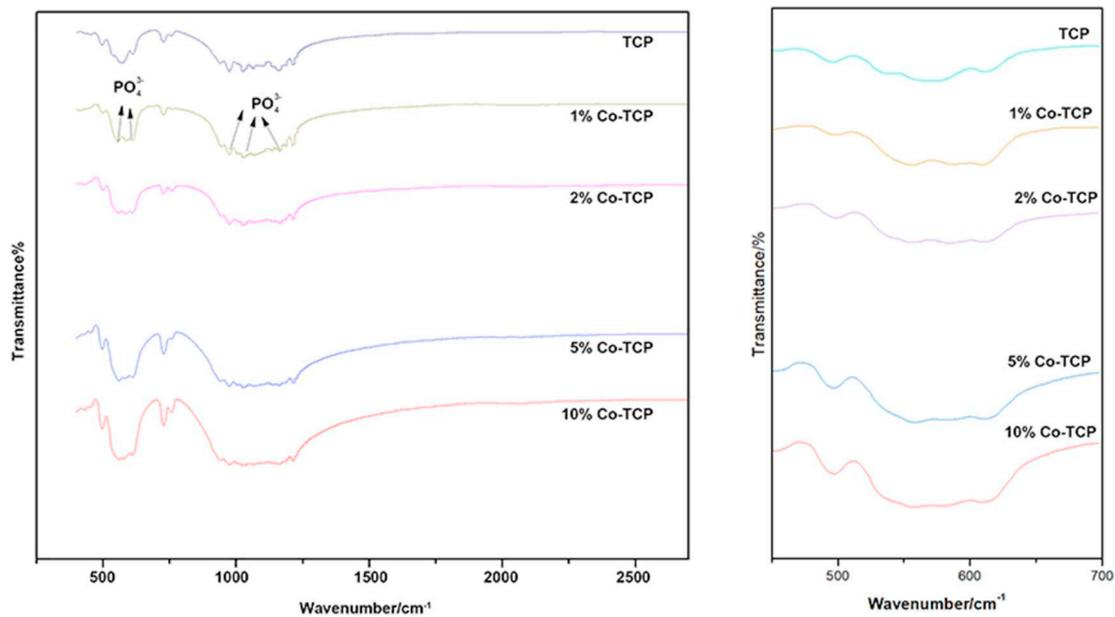
Fig. 4. The FT-IR spectra of Co-TCP with different concentrations of Co. The presence of phosphate is marked and the zoom picture in the range of 450 to 700  $\text{cm}^{-1}$  was shown in the right panel.
