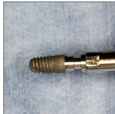
**Fig. 5.** Photograph of the Ta-coated SLA implant. Ta coatings were successfully prepared using VPS. The thread-form structure of the implant surface was still clearly visible.
