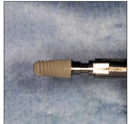
**Fig. 1.** Photograph of SLA implant before Ta coating. The implants had slightly tapered bodies with an outer diameter of 4 mm and a length of 8 mm. The surface was obtained after SLA treatments. They were designed and manufactured as substrates for the preparation of Ta-coated implants.
