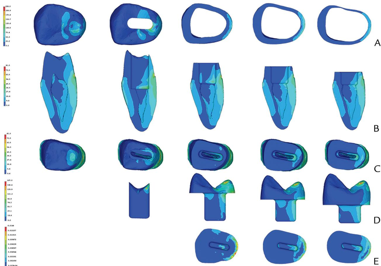
**Figure 3.** Von Mises stress distributions (MPa) in natural tooth and teeth restored with composite resin and endocrowns. A, Enamel. B, C, Dentin. D, Restoration and von Mises strain distributions of models E1, E2, and E3. E, Cement layer under oblique load of 200 N.
