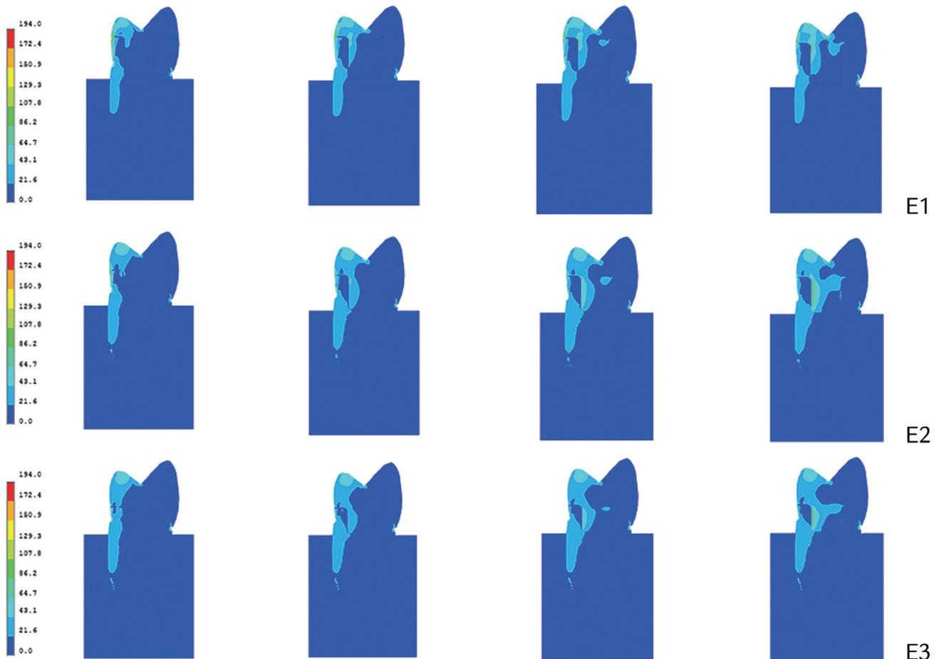
**Figure 4.** Von Mises stress distributions (MPa) in models E1, E2, and E3 in total under oblique load of 200 N.
