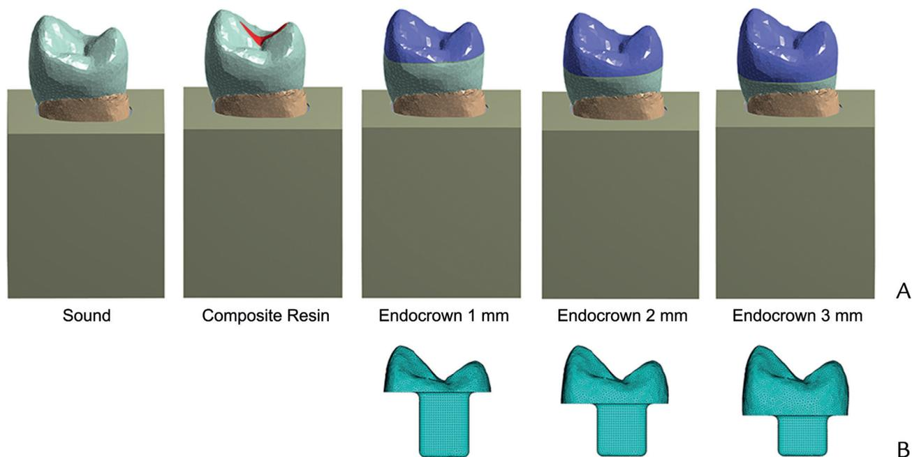
**Figure 1.** A, Finite element models of models S, R, E1, E2, and E3. B, Endocrown thicknesses for models E1, E2, and E3.
