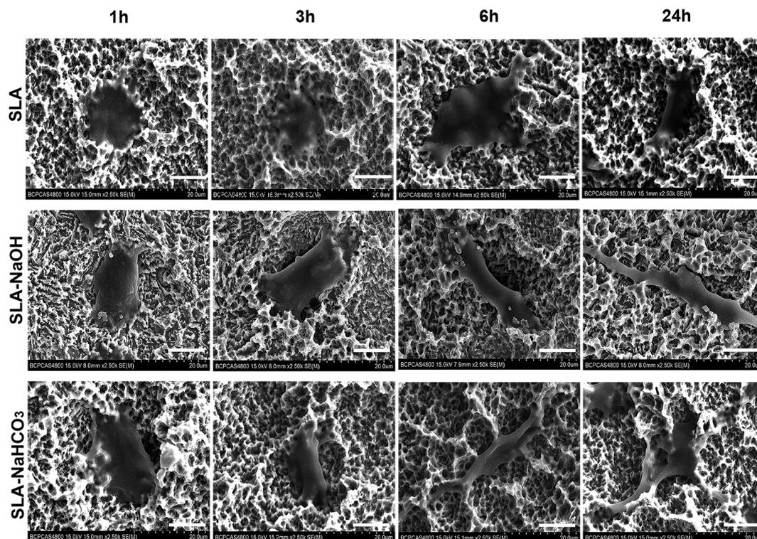
Fig. 6 SEM imaging for representative morphology of specimens with fixed MG63 cells on SLA, sodium hydroxide treated SLA and sodium bicarbonate treated SLA surfaces after 1 hour, 3 hours, 6 hours and 24 hours incubation. MG63 cells extended more lamellipodia and filopodia than that on the untreated SLA surface at the time point of 1 hour, 3 hours and 6 hours, no morphological differences were observed at the later time of 24 hours. Scale bar = 10  $\mu\text{m}$ .
