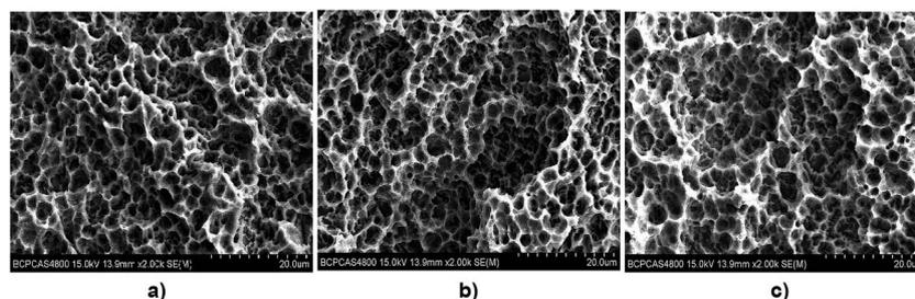
Fig. 1 SEM images of the SLA (a), sodium hydroxide treated SLA (b) and sodium bicarbonate treated SLA (c) surfaces. All the surfaces showed the similarity in morphology and no distinguishable differences on SEM imaging.
