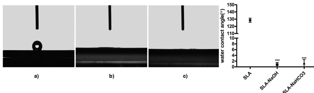
Fig. 2 Water contact angle measurements of SLA surface (a), sodium hydroxide (b) and sodium bicarbonate treated SLA (c) surfaces. After the alkaline treatments, both of the sodium hydroxide treated SLA (b) and sodium bicarbonate treated SLA (c) became superhydrophilic ( $\sim 0^\circ$ ) ( $***p < 0.001$  when compared with SLA,  $n = 4$ ).
