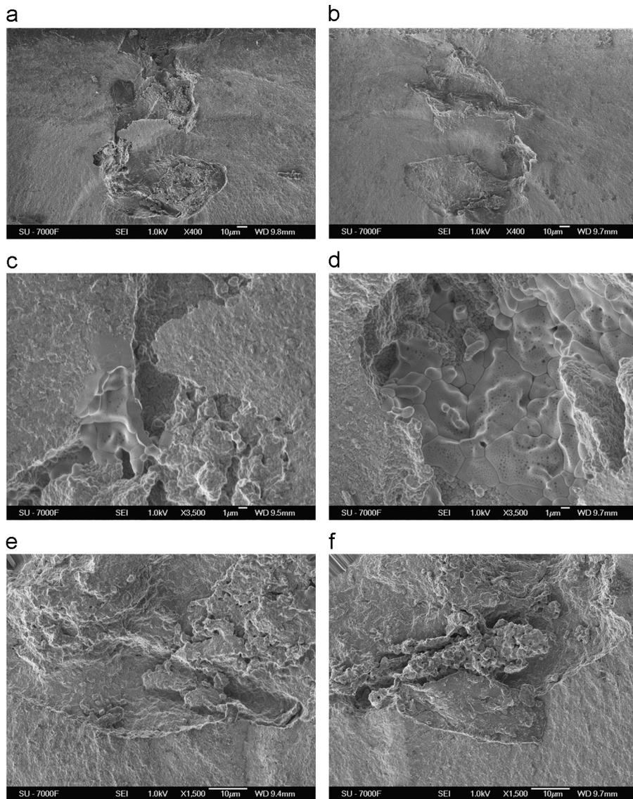
Fig. 4. SEM micrographs revealing the microstructure of a pair of fracture surfaces taken on a bi-colored sample that failed at the color gradient zone during bending test. The twist hackle markings point to the fracture origin in (a) and (b). Irregular grains with porous surfaces (c,d), large voids and critical agglomerates (e,f) are seen as common defects.
