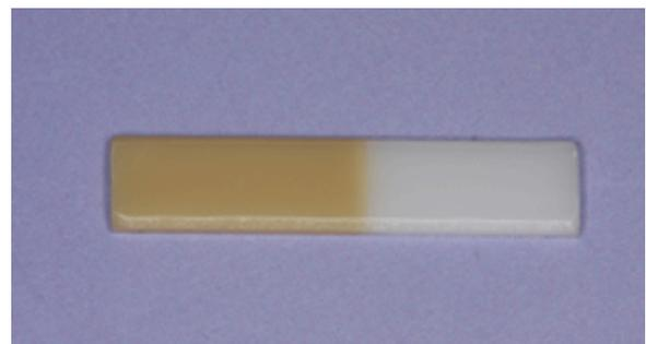
Fig. 1. A photo showing a 20 mm long bi-colored zirconia test bar prepared for four-point bending test.
