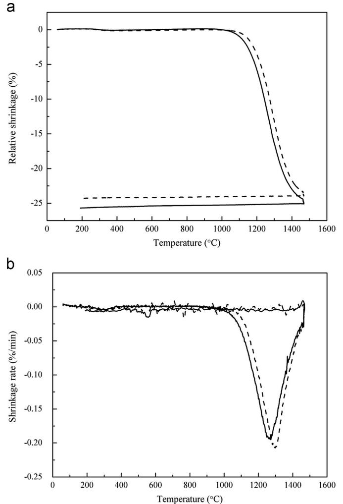
Fig. 2. Dilatometer curves illustrating the sintering properties of the two zirconia powders, TZ-3YSB-E (dash line) and TZ-YELLOW-SBE (solid line), yielding white and yellow color, respectively. The direct measured linear shrinkage versus temperature in (a) and calculated densification rate versus temperature in (b).
