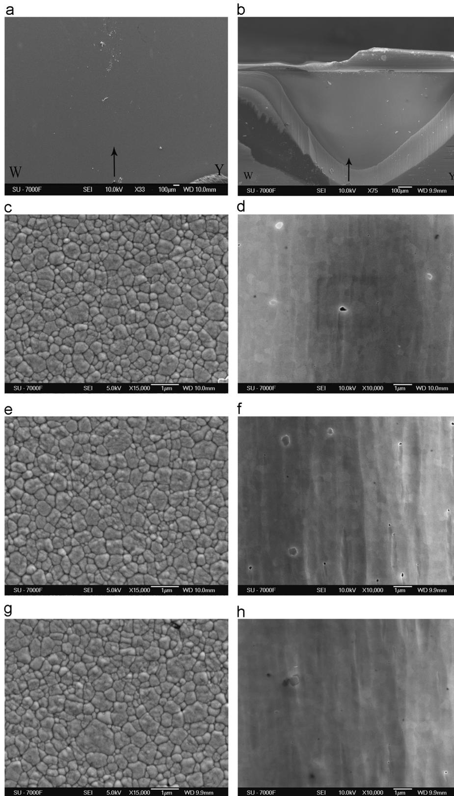
Fig. 3. SEM micrographs showing the microstructure of the bi-colored zirconia ceramics. Low magnification images of the polished surface (a) and cross-section (b) revealing the overall homogeneity of the sample. High magnification images of the polished surface and cross-section taken on the white region (c,d), color gradient zone (e,f) and yellow region (g,h), respectively.
