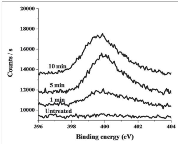
**Figure 3.** X-ray photoelectron spectroscopy (XPS) analysis of the nitrogen content of PLLA nanofibers before and after plasma treatment.
