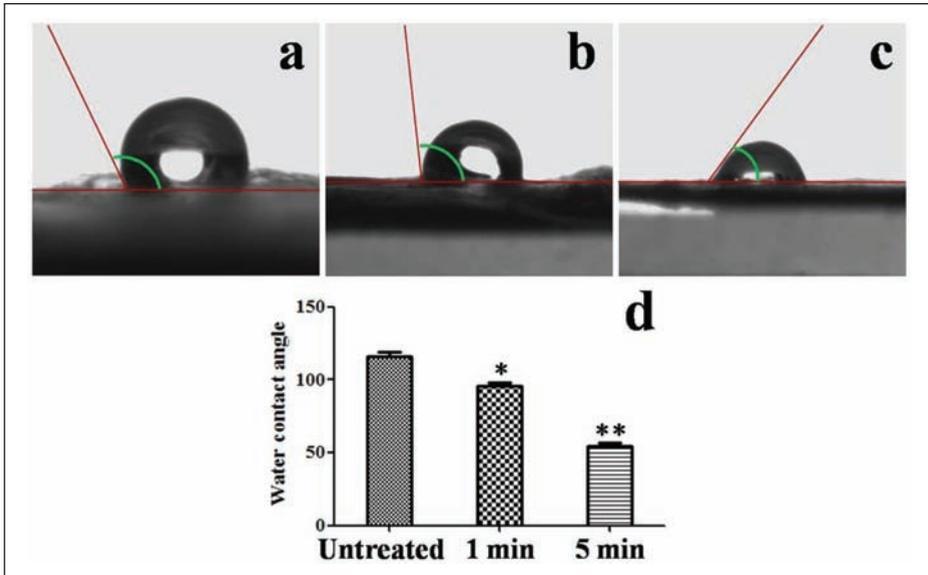
**Figure 2.** Typical water droplet images of distilled water 5 s after being dropped onto an (a) untreated or plasma-treated PLLA nanofibers surface for (b) 1 and (c) 5 min. (d) The water contact angle measured from the indicated samples ( $n = 30$ ).
