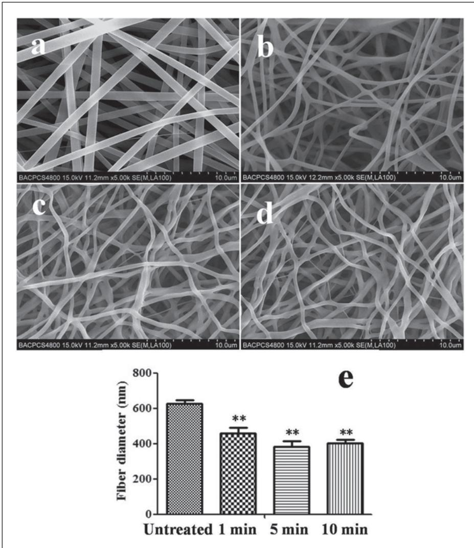
**Figure 1.** SEM images of (a) untreated PLLA nanofibers and plasma-treated for (b) 1, (c) 5, and (d) 10 min. (e) The fiber diameter (nm) of untreated and plasma-treated nanofibers ( $n = 100$ ).
