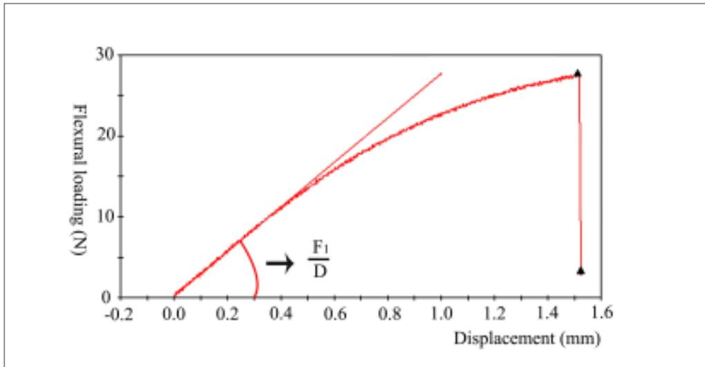
**Fig 1** Representative load-deflection graph used to calculate the flexural modulus. This specific sample is the composite with 50 wt% filler content.
