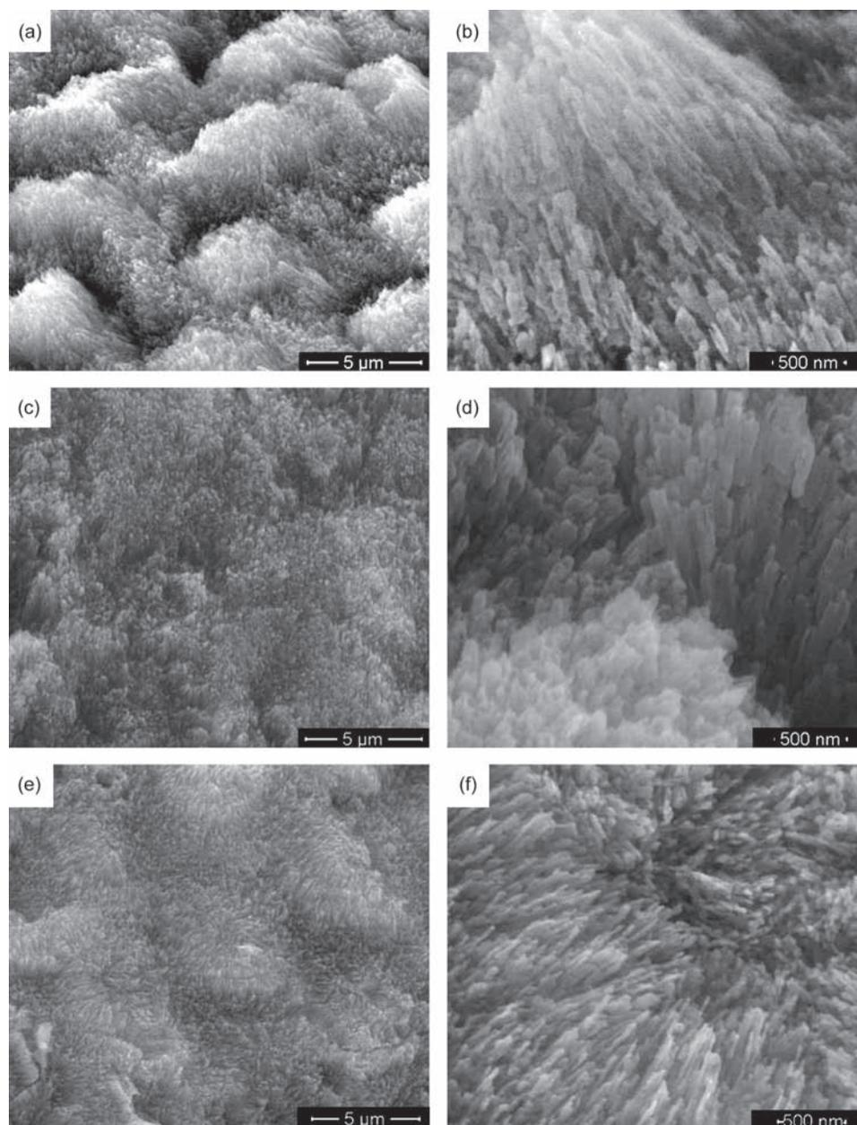
**Fig. 4.** SEM images of enamel surfaces treated by *n*-FA pastes under different conditions: pH < 1 (a), (b), pH = 4.5 (c), (d) and pH = 7.5 (e), (f).
