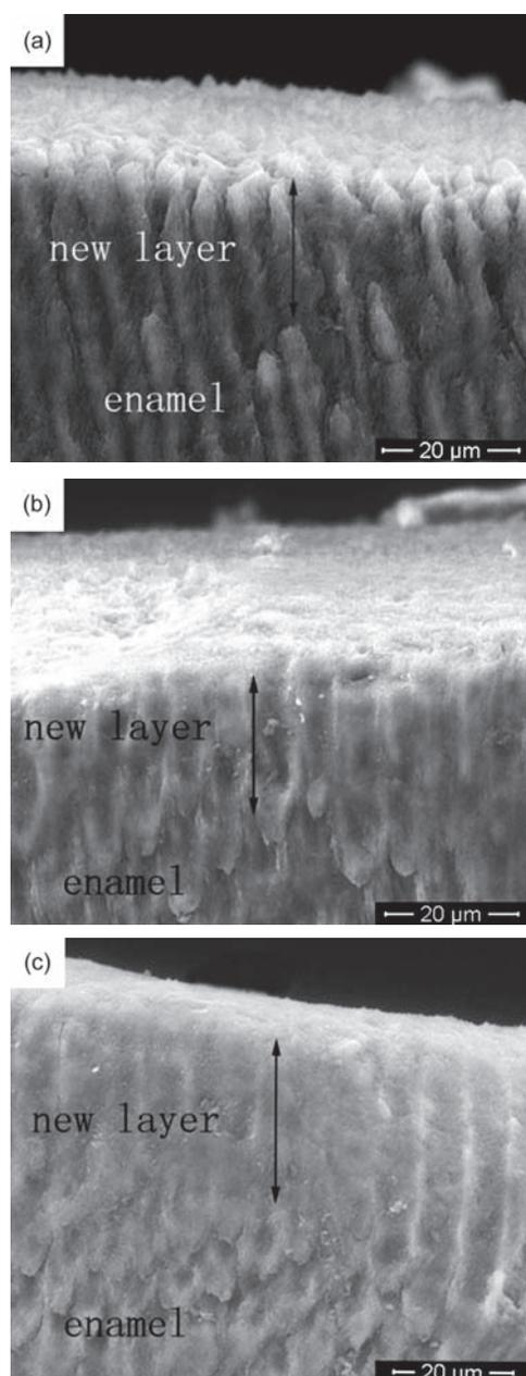
**Fig. 5.** SEM images for the cross-section of enamel treated by the *n*-FA pastes under different conditions, (a): pH < 1, (b): pH = 4.5 and (c): pH = 7.5.
