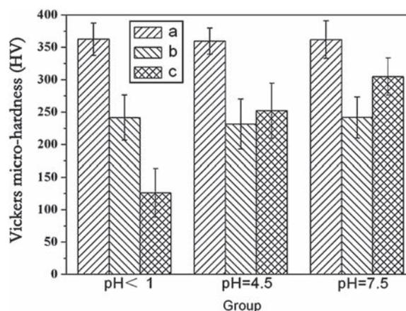
**Fig. 8.** Vickers micro-hardness of the enamel surfaces before and after treatments with the *n*-FA pastes at different pH conditions, (a): before acid pretreatment, (b): after acid pretreatment, and (c): after formation of new layers.
