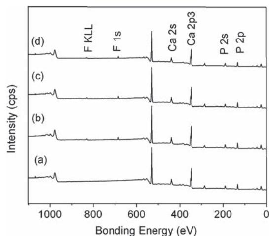
**Fig. 6.** XPS of dental enamel surfaces before (a) and after treatment with *n*-FA pastes at different pH conditions: pH < 1 (b), pH = 4.5 (c) and pH = 7.5 (d).
