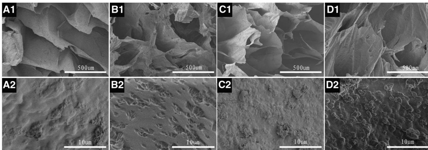
Fig. 1. SEM images of gelatin/CM-chitosan/ $\beta$ -TCP composite scaffolds fabricated with ultrasonic time of (A) 5 min, (B) 20 min, (C) 50 min, and (D) 2 h. The  $\beta$ -TCP fraction was 30%.
