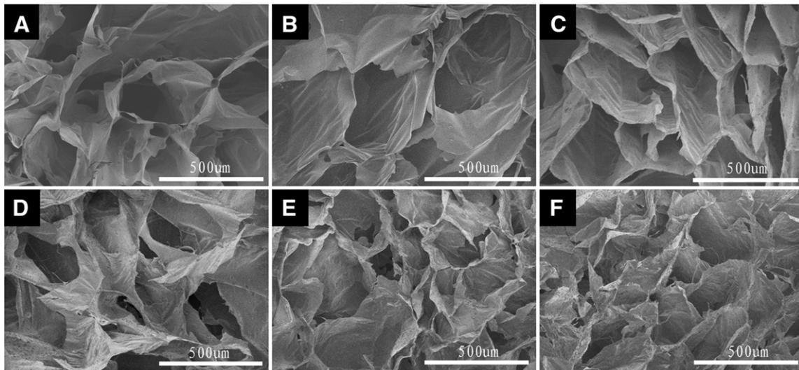
Fig. 2. SEM images of gelatin/CM-chitosan/β-TCP composite scaffolds with β-TCP fraction of (A) 0%, (B) 5%, (C) 10%, (D) 20%, (E) 30%, and (F) 40%. The ultrasonic time was 20 min.
