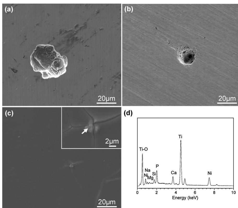
Fig. 5. SEM surface morphologies of (a) CG NiTi, (b) UFG NiTi without SrO–SiO<sub>2</sub>–TiO<sub>2</sub> sol–gel coating and (c) UFG NiTi with SrO–SiO<sub>2</sub>–TiO<sub>2</sub> sol–gel coating after electrochemical tests, with the high-magnification image as the inset on the upper-right corner, (d) EDS spectrum from the position marked by an arrow in the inset figure of (c).
