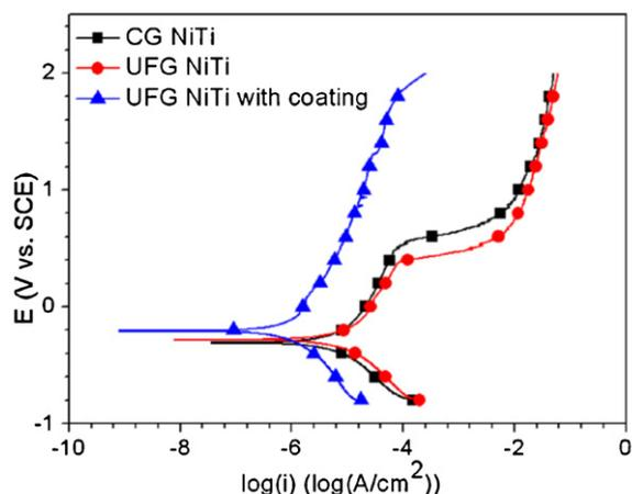
Fig. 4. Potentiodynamic polarization curves of CG NiTi and UFG NiTi with and without SrO–SiO<sub>2</sub>–TiO<sub>2</sub> sol–gel coating.
