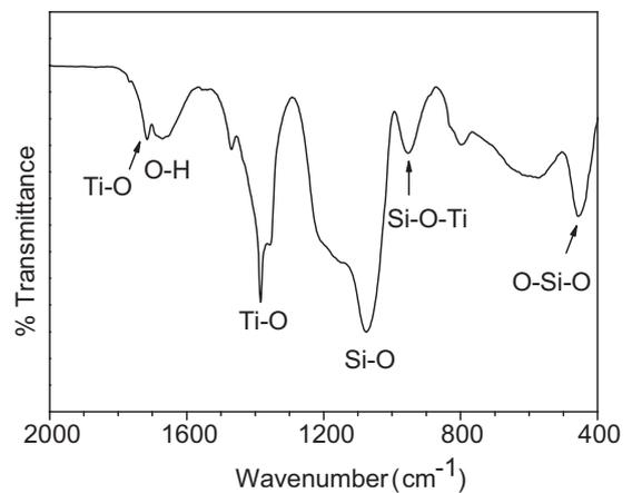
Fig. 3. FTIR spectrum of powders of dried SrO-SiO<sub>2</sub>-TiO<sub>2</sub> gel with subsequent hydrothermal treatment.
