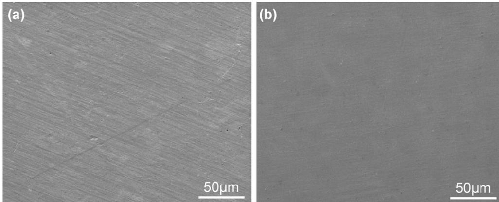
Fig. 1. SEM surface morphologies of UFG NiTi before (a) and after (b) SrO-SiO<sub>2</sub>-TiO<sub>2</sub> sol-gel coating.
