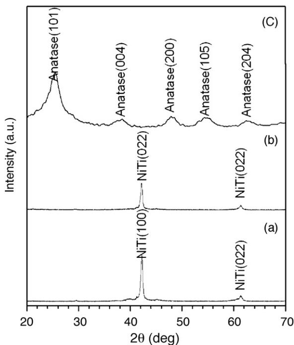
Fig. 2. XRD profiles of (a) UFG NiTi, (b) UFG NiTi with SrO-SiO<sub>2</sub>-TiO<sub>2</sub> sol-gel coating and (c) powders of dried SrO-SiO<sub>2</sub>-TiO<sub>2</sub> gel.
