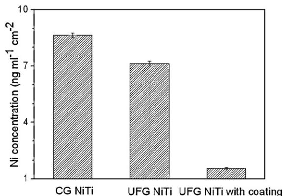
Fig. 7. The release of Ni ions of CG-NiTi and UFG-NiTi with and without SrO–SiO<sub>2</sub>–TiO<sub>2</sub> sol–gel coating.
