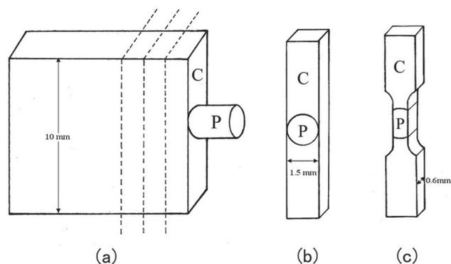
Fig. 1 Schematic illustration of specimens making for microtensile test (C: cement, P: fiber post). (a) The resin slab which was 10 mm in width contained the fiber post in the center. (b) The resin slab was sectioned vertically to the post to obtain resin beams, diameter of the fiber post is 1.5 mm. (c) The resin beam was trimmed into dumbbell-shaped specimens to expose the post surface, thickness of the specimens is about 0.6 mm.
