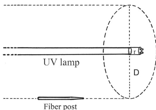
Fig. 4 Schematic illustration of UV irradiation. The UV irradiation energy on the post surface can be calculated according to the following formulas.  $I = w / [2\pi \cdot (r + D) \cdot L]$ ,  $E = I \cdot t$ . ( $I$ =irradiation intensity on post surface,  $E$ =UV irradiation energy on post surface,  $w$ =lamp power,  $r$ =radius of the UV lamp,  $D$ =distance between lamp and fiber post,  $L$ =length of the UV lamp,  $t$ =irradiation period).
