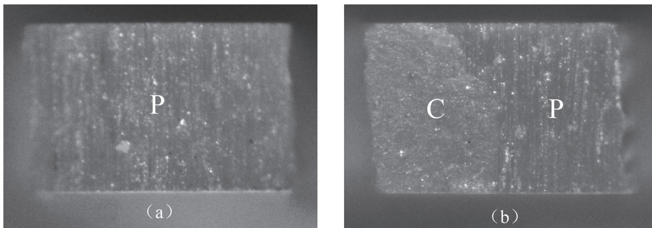
Fig. 3 Representative micrographs of the failure modes evaluation under the stereomicroscope at 80× magnification (C: cement, P: fiber post). (a). Adhesive failure displayed solely the impression of the fiber post surface over failure area. (b) Mixed failure displayed both the impression of the post and residual resin cement.
