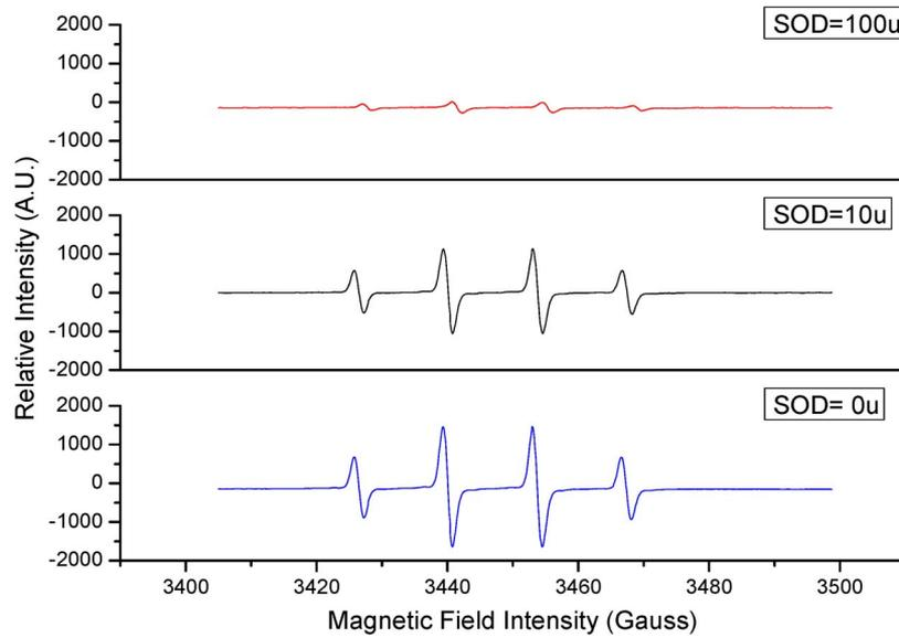
Fig. 6. DMPO-OH signals at different SOD concentrations.
