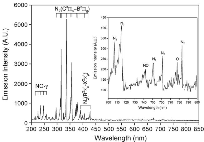
Fig. 8. OES (from 200 to 850 nm) of the PMJ in air. Inset shows the emissions in the near-infrared section from 700 to 800 nm.
