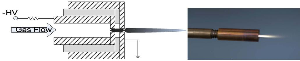
Fig. 1. (a) Schematic diagram. (b) Picture of PMJ.
